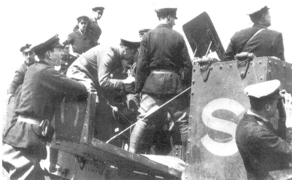
29: The crew of a Seabrook armoured lorry in action. This clearly shows how the armoured sides of the body folded down to allow the gun to traverse 360°. Not all guns were fitted with a shield like this one. Via Laurie Milner (IWM HU 66661)
