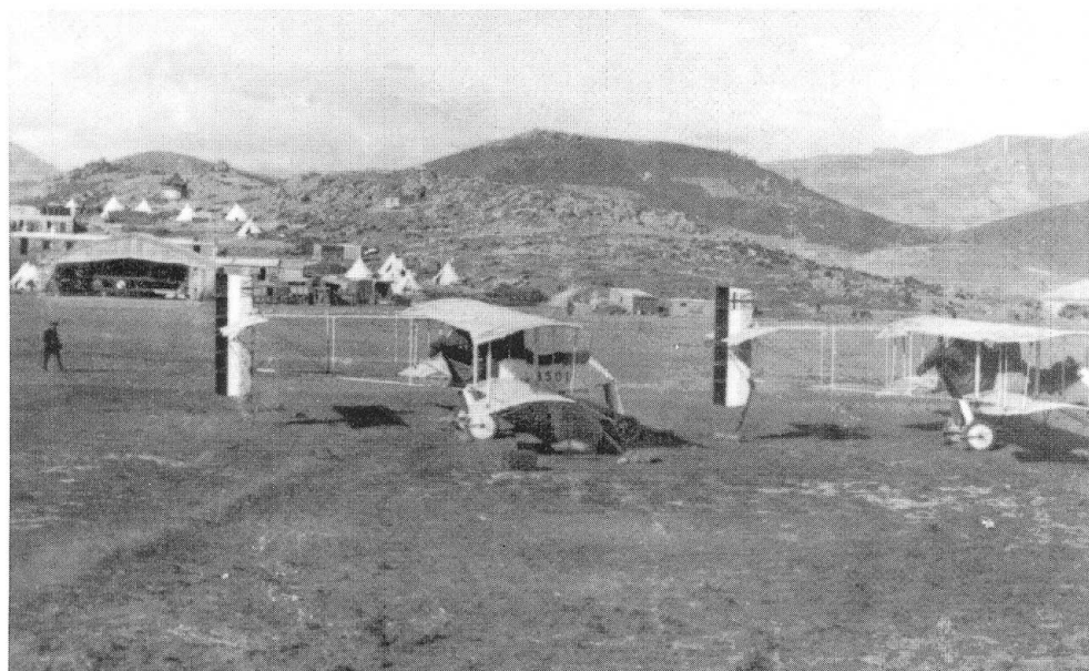
94: Two Voisin L.A.S bombers, Nos. 8501 and 8503, probably of 3 Wing at Imbros in summer 1915. 8501 was written off in early 1916, while 8503 force landed in a salt lake on 17 January 1916. Note how the early Union Jack markings on the rudders have been supplemented by stripes (Barry Ketley)
