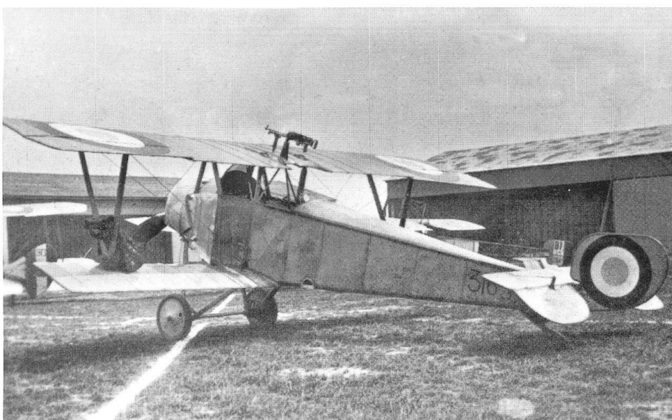
146: The first Nieuport 10 delivered to the RNAS, number 3163 arrived at Naval 1 (which became 1 Wing RNAS) at St. Pol in late May 1915. It was written off by December that year. All 24 of the first batch delivered retained their French cockades above and below the wings and bore additional markings on the rudder surfaces, as required by the RFC from November 1914. The tail of a B.E.2c, 973, shows to the left. Behind 3163 is Bleriot XI-BG parasol 1547. This machine served with Naval 1 for precisely three months between 21 March until 21 June 1915 (Barry Ketley)
