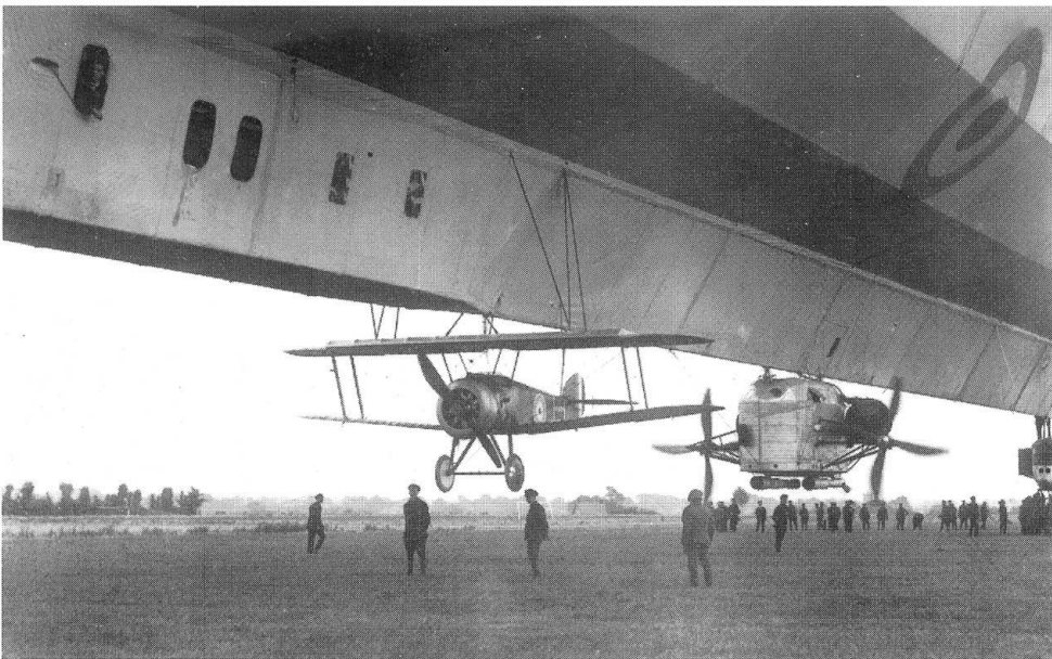
196: The six machines of the R23X class provided platforms for a number of interesting experiments. Here R23 is seen at Howden with Sopwith Camel N6814 suspended beneath her. These 'drop' trials were fairly successful, having been conceived as a way of getting a fighter up to the same altitudes as a Zeppelin and therefore able to attack it more effectively. Earlier experiments along these lines using SS type airships were abandoned after the deaths of Cdr. Osborne and Lt. Cdr. de Courcy Ireland (IWM Q 27476)
