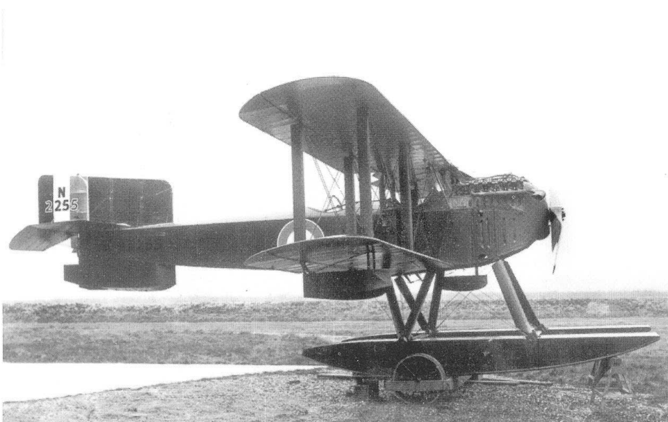
273: The first examples of what was to become a very long-lived line of aeroplanes were just entering service with the Royal Navy as the war ended. Originally built as a Fairey IIIB, N2255 was converted to a IIIC by the substitution of a Rolls-Royce Eagle engine in place of the Sunbeam Maori. Regarded as probably the best floatplane of the 1914-1918 war, it was the first general-purpose aircraft for the RNAS, combining the dual roles of bombing and reconnaissance. This one was converted to civil use as G-EAPV and later went to Sweden (Barry Ketley)
