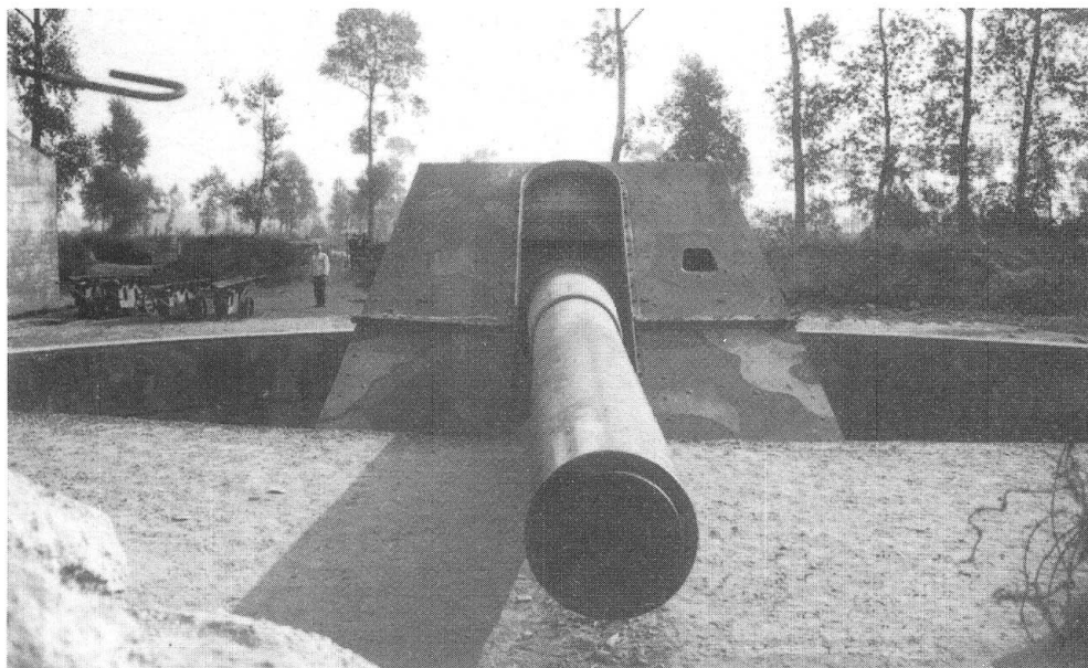
222: Seen immediately post-war, this is one of the heavy guns which the Germans used to both shell the RNAS airfields on the Flanders coast and also to dissuade naval forces from approaching too close to the German-held ports used by the U-boats. Nicknamed the 'Leugenboom', it is a 380 mm turreted cannon, one of a battery at Breedene just to the east of Ostend, which was used to shell Dunkirk. Targets like this were attacked by RNAS bombers in support of the naval raids on Zeebrugge and Ostend in late April 1918. The man in the background to the left of the gun gives an indication of its size (Barry Kelley)
