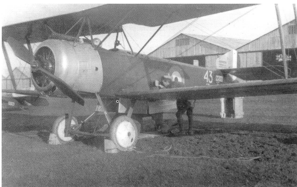
149 Right: Sopwith 1 1/2 Strutter N5116 arrived at Luxeuil on 15 November 1916. Seen here as a single-seat bomber, number '43' served with 4 Flight, then 2 Squadron of 3 Wing before being transferred to the French. Powered by a 110hp Le Rhone engine, the 1 1/2 Strutter was the first British aircraft to have a factory-fitted synchronised machine gun for the pilot. Versatile and easy to fly, the machine quickly earned a reputation second to none as a bomber, fighter escort and reconnaissance aircraft and served in every theatre (IWM 868078)
