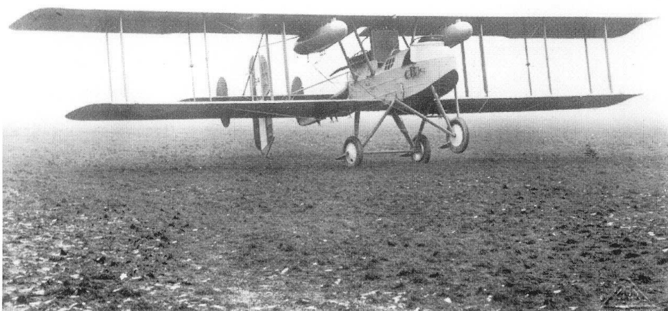
140: This is believed to be a Grahame-White built Breguet Type 5, possibly 9426, with a 250hp Rolls-Royce engine. One of a small batch of ten, known by the manufacturer as a Grahame-White Type XIX, and intended for 3 Wing at Luxeuil, it was obsolete by the time it was completed in late 1916. Consequently it was delivered to Hendon (where this picture may have been taken) and never saw service (Barry Ketley)
